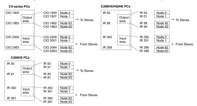
Each node address is allocated one input and one output word starting from node 00. If a Slave requires more than one input or one output word, then it is assigned more than one node address. If a Slave requires less than one word, it simply uses the rightmost bits in the word allocated to it.
